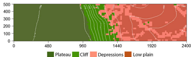
Figure 3. Topographic map of the Mpala 120-ha (2400 × 500 m) plot with 10-m contour interval and overlay of the four topographic habitats defined in the study, based on altitude, slope and convexity.
