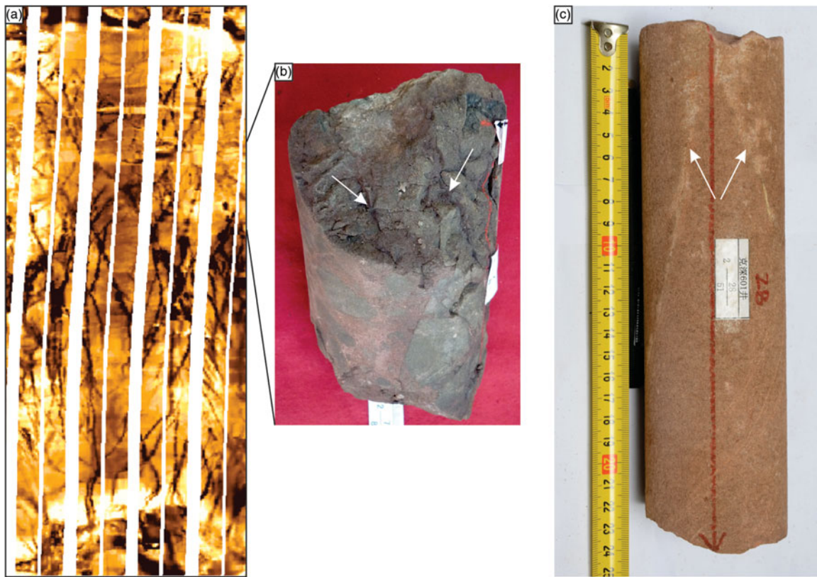
Fig. 11. (colour online) Conjugate fracture pairs in the borehole image and cores. (a) The processed electrical image having two sets of fractures with the opposite dip-directions. (b) Core pieces with conjugate fracture pairs, calibrated to the corresponding borehole image; the core shift process can be seen in Nian et al. (2016). (c) Two sets of conjugate fractures in the core; the white staining along the fracture traces suggests that fractures are serving as conduits to fluid flow.
