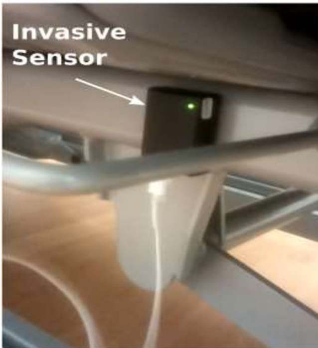
Fig. 3. Invasive device sensor flashing the green light when HCW manipulates the invasive device.
