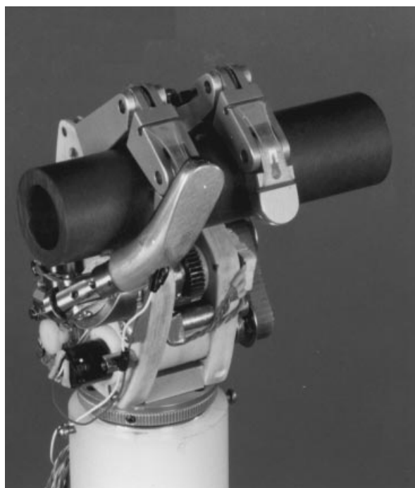
Fig. 3. The Oxford Intelligent Hand prosthesis in power grip. This grip form is not possible with conventional devices.
