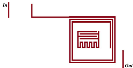
Fig. 3. Resonators used in simulations: one spiral and the other including a meander line, used separately or together.
