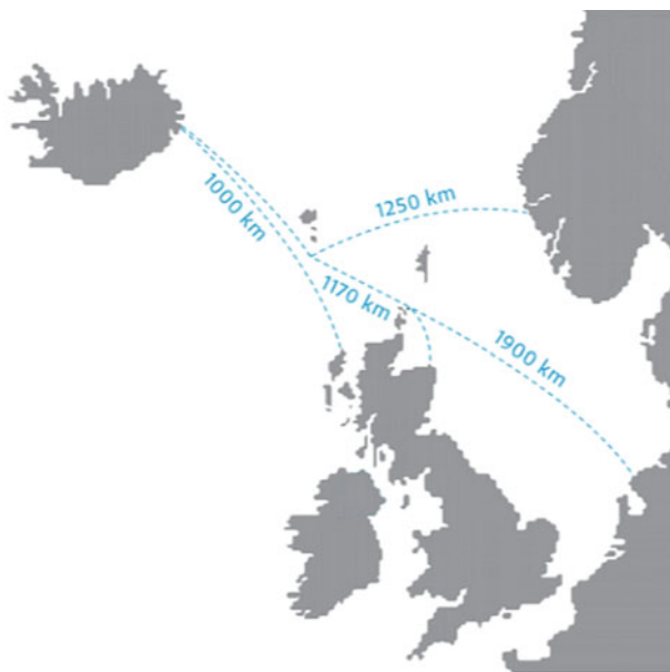
Fig. 2. Possible connections of submarine cable between Iceland and Europe. Source: Landsvirkjun 2013.
