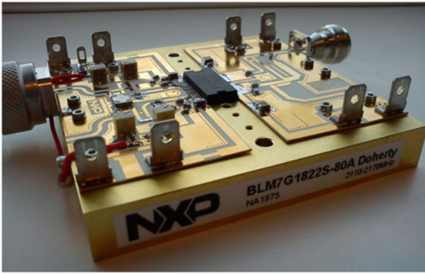
Fig. 10. Photograph of the test board for the asymmetric Doherty MMIC.
