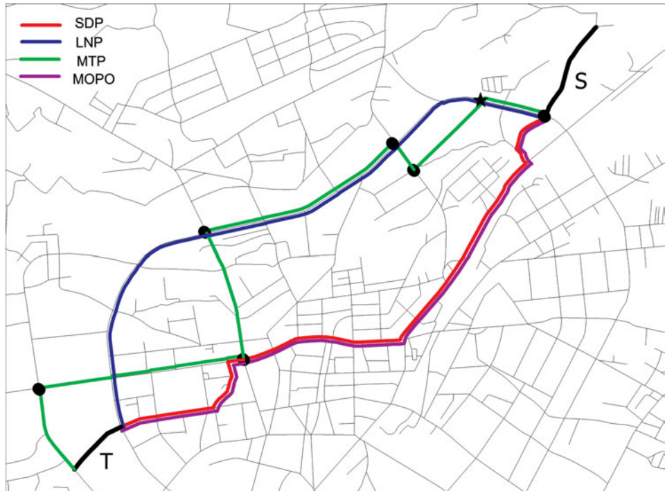
Figure 7. The optimal paths of SDP, LNP, MTP and MOPO problems in a radial-circumferential road network.
