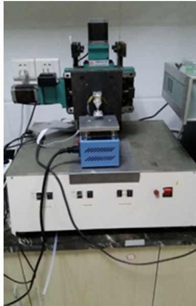
Figure 7. The home-made tribometer for adhesive material test.
