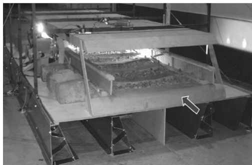
Figure 13. Wind tunnel tests on full scale track bed (36) .
