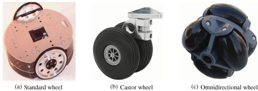
Fig 1. (Colour online) Schematic view of various wheel types used in mobile robots.
