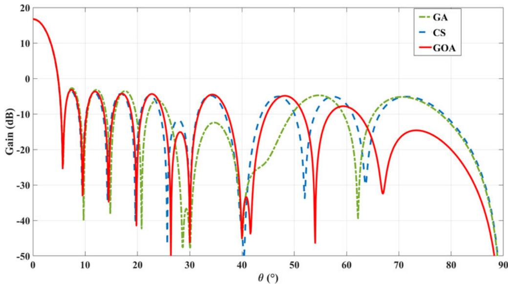
Fig. 3. The comparisons of the radiation pattern performances in the excitation amplitudes optimization.
