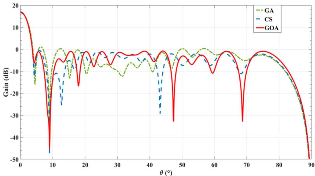
Fig. 4. The comparisons of the radiation pattern performances in the excitation phases optimization.
