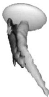
FIGURE 2. Isosurfaces of streamwise vorticity in the two-threaded wake behind a spiralling bubble; from the numerical simulation by Mougin & Magnaudet (2002).
