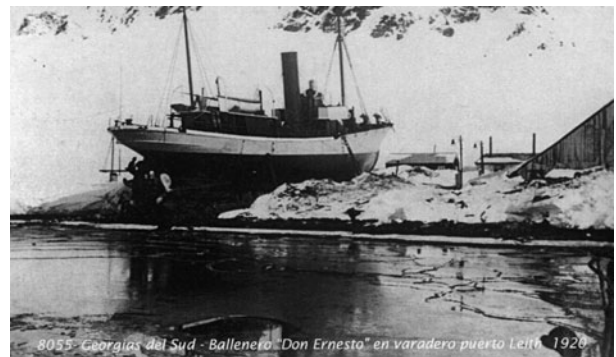
Fig. 5. The whale catcher Don Ernesto , owned by Compania Argentina de Pesca , built in 1910 of steel construction with an ice-strengthened hull. Her tonnage was 221 tons, displacement unknown, length 38 m and combined power from two engines of 700 hp.
