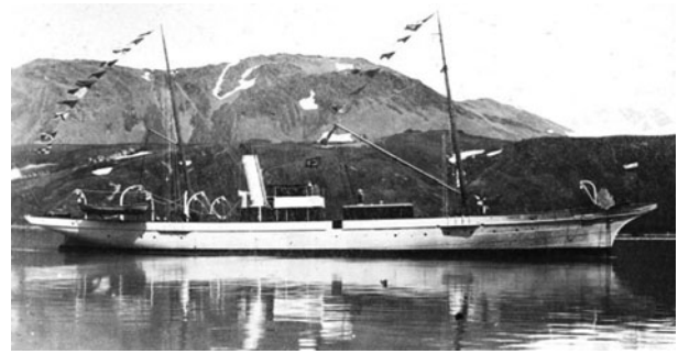
Fig. 4. The steam yacht Undine , owned by Compania Argentina de Pesca , built in 1884 of iron construction. Her tonnage was 338 tons, displacement unknown, length 50 m and power 400 hp.
