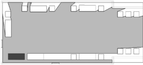
Fig. 30. The visibility space of the lower left display cabinet derived by DSIm.
