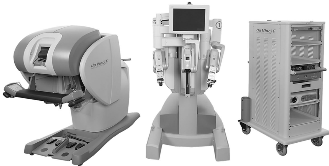
Fig. 1. Components to the da Vinci SHD system: (from left to right) console, patient side cart, stack system. (Courtesy of Intuitive Surgical).
