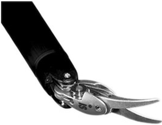
Fig. 3. The instruments used by the da Vinci system have endowrists which allow 7 degrees of freedom in manipulating the instrument. (Courtesy of Intuitive Surgical).
