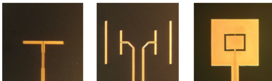
Fig. 15. Photographs of different antennas realized in the RDL of the eWLB package: dipole (left), array of two dipoles with reflectors (center), and CPW patch (right).
