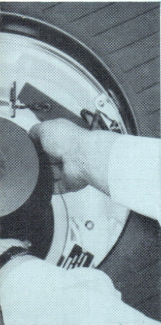
The rotor of the M.S.E. high speed centrifuge is forged by H.D.A. in a titanium alloy.
