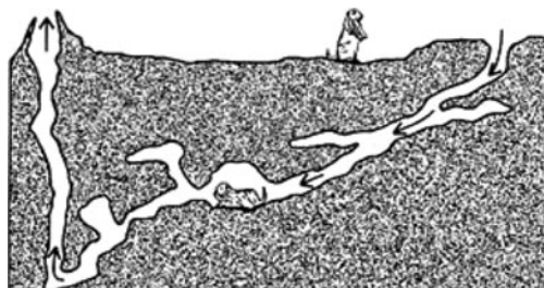
Fig. 3. A prairie dog den has heightened entrances and flat entrances. When the wind is blowing, the static pressure over the heightened entrances decreases, causing ventilation inside the den. Adapted from “Wind-induced ventilation of the burrow of the prairie-dog, Cynomys ludovicianus ,” by S. Vogel, C.P. Ellington, and D.L. Kilgore, 1973, Journal of Comparative Physiology 85A(1), 1–14. Copyright Springer Science+Business Media 1973. Adapted with permission.
