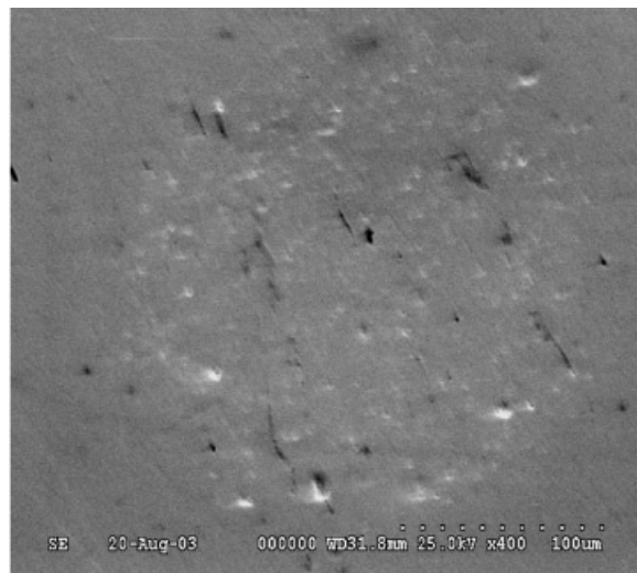
Fig. 5. SEM Micrograph of irradiated Cu surface at magnification \times 400 showing the damaged circular region of radius 114.28 \mu\text{m} , which is also due to forward peaking.
