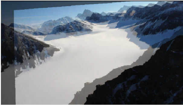
Fig. 6. Comparison of two images taken by the same camera, before and after maintenance sessions yielded camera motion. Since the camera lens is still positioned at the same point after putting the camera back on its holder, a 2D second-order polynomial distortion is used to associate far-away (ridge, fjord) and nearby stable (rock) features in order to provide a consistent dataset over the 4 year acquisition period. All images must be centered identically for the reference points located on the field and on a reference image to be applicable.
