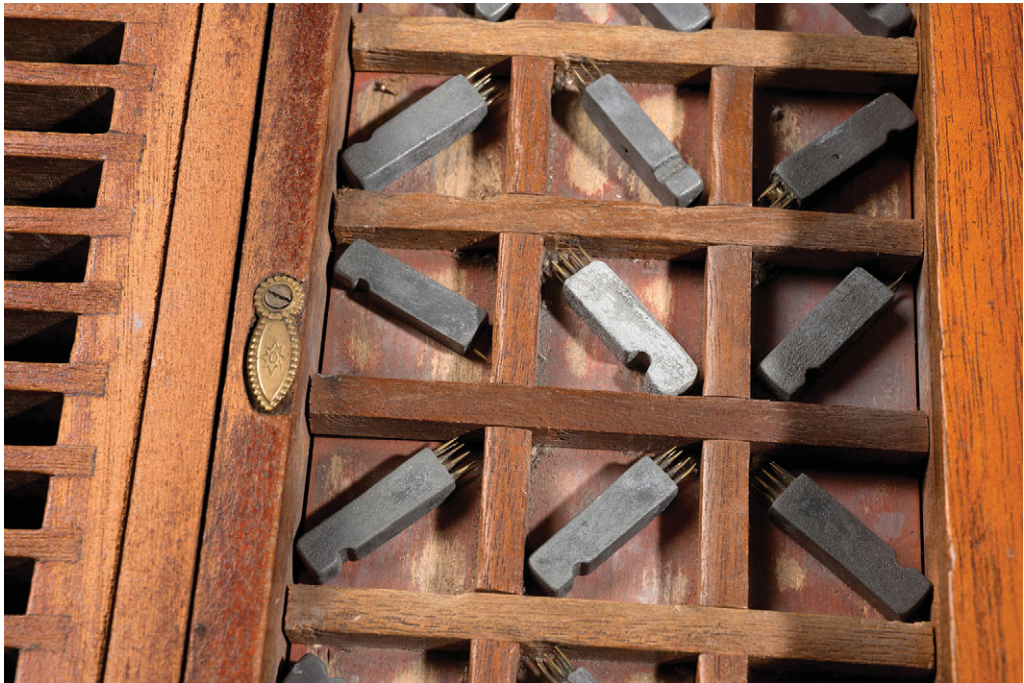
Figure 18. (Color online) Klein Type Box, c. 1840. Folding box, green felt backing to type board, 24 lines, lead type. With key and catches. Courtesy of RNIB Collection.
