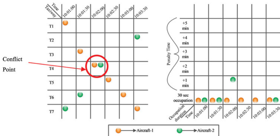
Figure 11. (Colour online) An illustrative example of conflict detection in the mapping database.
