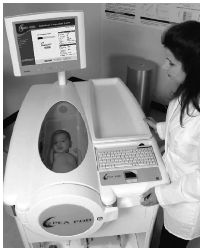
Fig. 1. PEA POD with an infant in the test chamber and an operator observing the infant’s behaviour and the progress of the measurement on the display monitor. (Photograph courtesy of COSMED USA Inc., reproduced with permission.)
