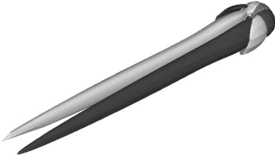
FIGURE 18. The asymmetric wake of the Ar = 0.6 ring following the mode I transition at Re = 130 . The ring is located at the top right-hand corner of the frame, and the flow direction is from the top right to the bottom left. Light and dark isosurfaces show negative and positive streamwise vorticity, respectively. Note the double-threaded wake structure, similar to the classic sphere wake.
