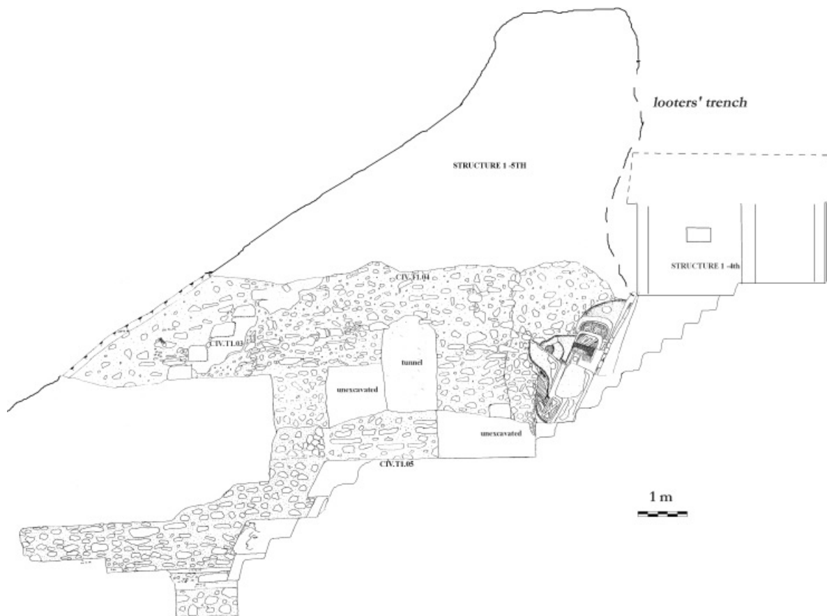
Figure 7. Stratigraphic profile of Structure I showing penultimate construction phase with stucco mask covered by last construction phase and damaged by looters' trench.
