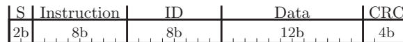
Fig. 3. Diagram showing the format for the 34-bit communication packet sent between capsules and between capsules and the control box. The packet contains 2 start bits (labelled S), an 8-bit instruction code, 8-bit ID code, 12-bits of data and a 4-bit CRC code.
