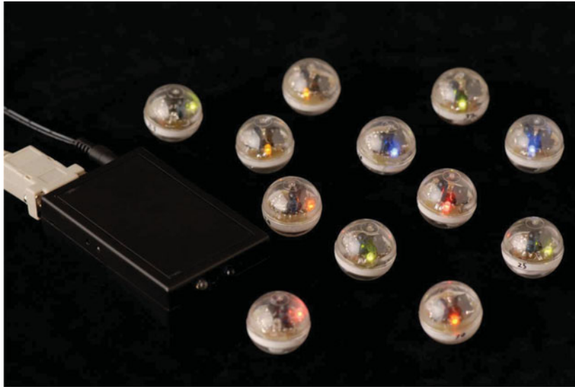
Fig. 1. Photograph of the group of 12 capsules and a control box that interfaces to a PC via a serial link. Each capsule has its LED switched on.
