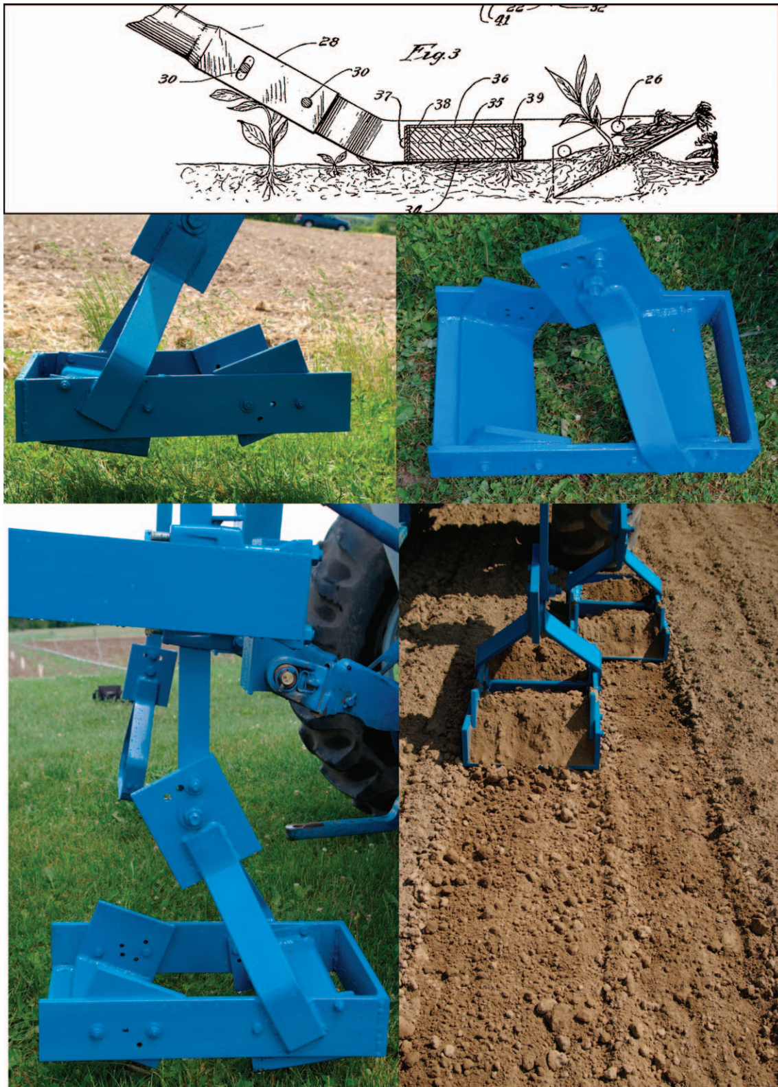
Figure 2. The block cultivator. Clockwise from top: original illustration of a hand tool designed in 1928 by M. Oakland; top-down view with the front of the cultivator to the right; rear view of soil disturbance after cultivation; side view showing the tool shank extending upward into a toolbar clamp and the toolbar attached to a tractor via a three-point hitch; side view of block cultivator with the front of tool to the left.
