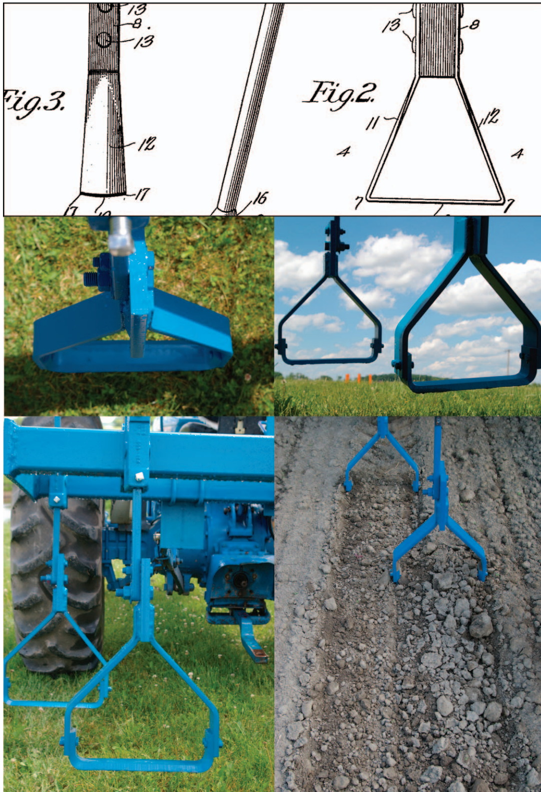
Figure 3. The stirrup cultivator. Clockwise from top: original illustration of a hand tool designed in 1903 by E. B. Morgan; front and side view; soil disturbance after cultivation; rear view of the cultivator where the tool shank extends upward into a toolbar clamp; top-down view.
