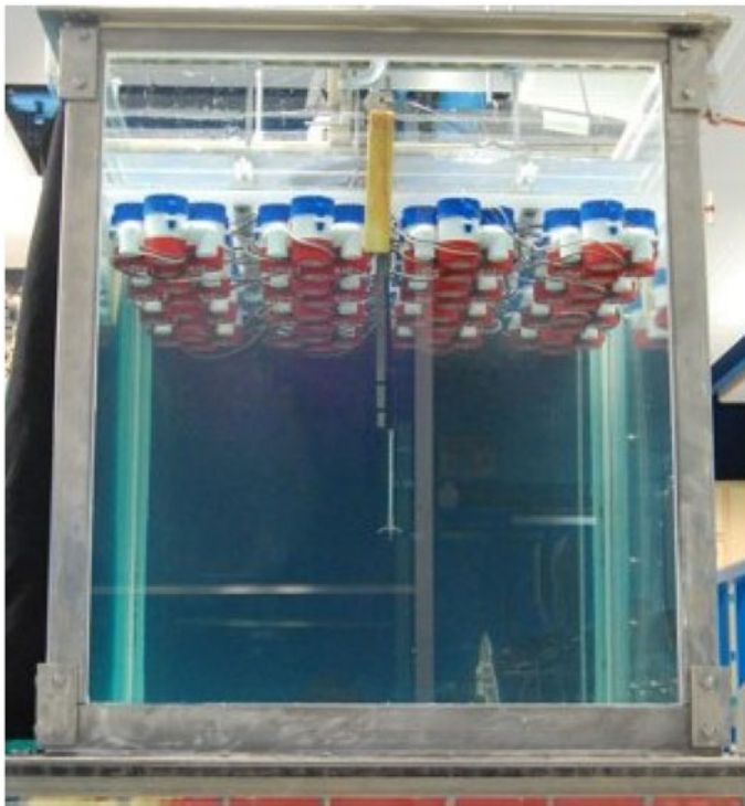
FIGURE 2. (Colour online) Photo of tank with the 8 \times 8 RASJA.
