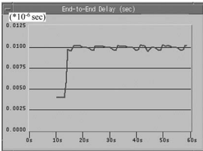
Fig. 8. Delay simulation of TCP with light traffic from a crane.
