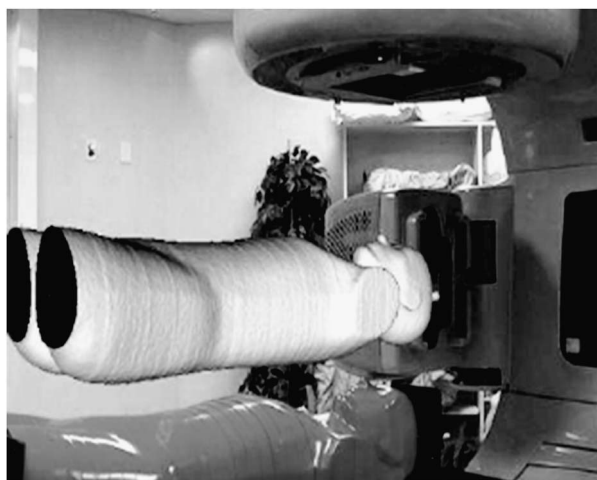
Figure 5. Body contour from CT scan (grey virtual image) and patient's true image (red anthropomorphic phantom). Reproduced with kind permission of Springer from Talbot et al. 16
