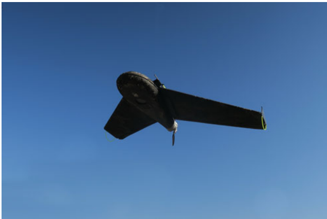
Fig. 2. The electrically-powered fixed-wing UAV "Ninox" used for the survey flights.
