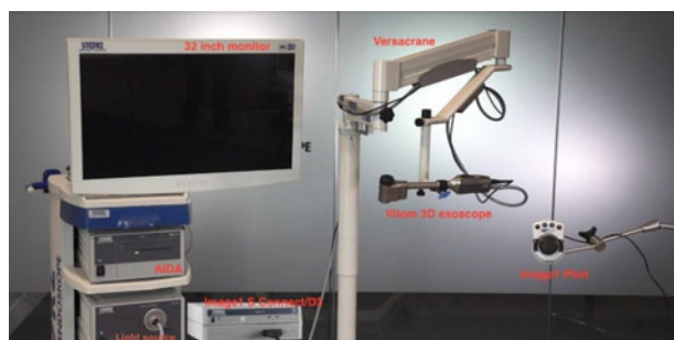
Fig. 1. Components of the Vitom 3D system (Karl Storz), with labels. AIDA = advanced image and data acquisition device
