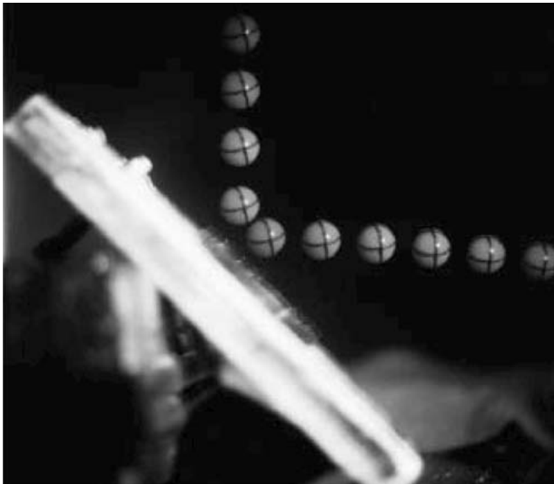
FIGURE 2. Sample picture of a nylon ball with a 0.0127 m diameter dropped from a height of 0.53 m onto a quartz disk inclined at an angle of 45^\circ to the horizontal and covered with a layer of oil of viscosity 0.975 \text{ kg m}^{-1} \text{ s}^{-1} and thickness of 80 \mu\text{m} , with the stroboscope running at 10 000 flashes per min.
