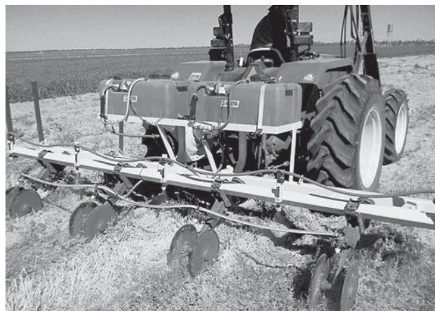
Figure 5. Applying Spray.Seed ® to bed surfaces and Glyphosate 450 ® to furrows in a single pass with the final version of the mulching implement ('Final design').
