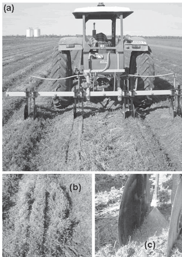
Figure 4. Applying Spray.Seed ® in a single pass with an intermediate stage ('Later stage') of the mulching implement. (a) Complete implement under field conditions. (b) Close-up of strip cut by coulters. (c) Close-up of coulters and nozzle.
