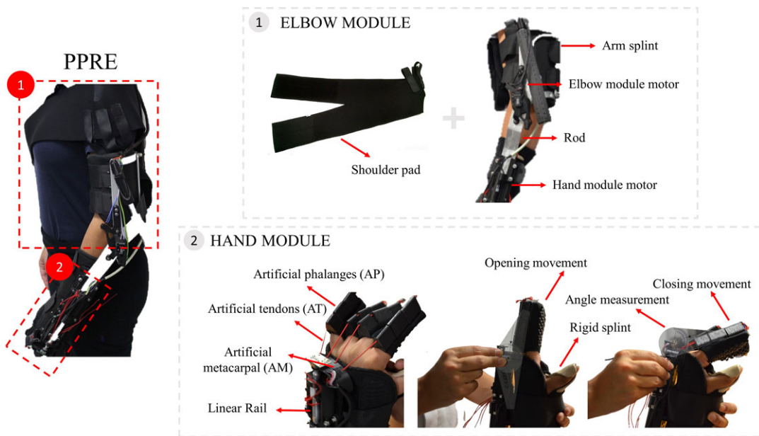
Figure 2. Pinotti Portable Robotic Exoskeleton (PPRE) hand module and elbow module.
