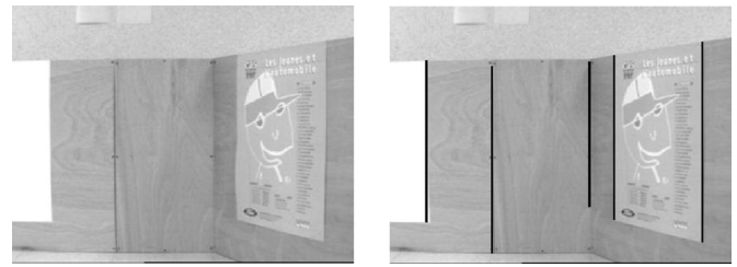
Fig. 8. Image of the camera and extracted vertical edges.
