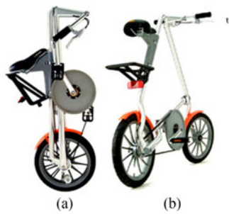
Fig. 5. (Color online) Strida folding bike. Images (of earlier model) used with permission ( http://www.strida.com ). (a) Folded state and (b) riding state.
