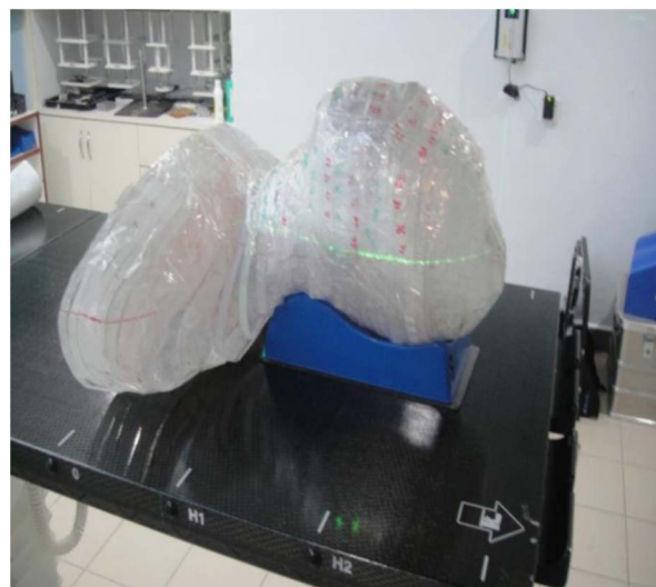
Figure 1. Fabricated anthropomorphic Perspex head and neck phantom for dosimetric verification of treatment delivery.
