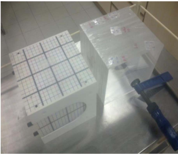
Figure 2. Head cube phantom (Scanditronix Wellhöver) and Perspex cube phantom.
