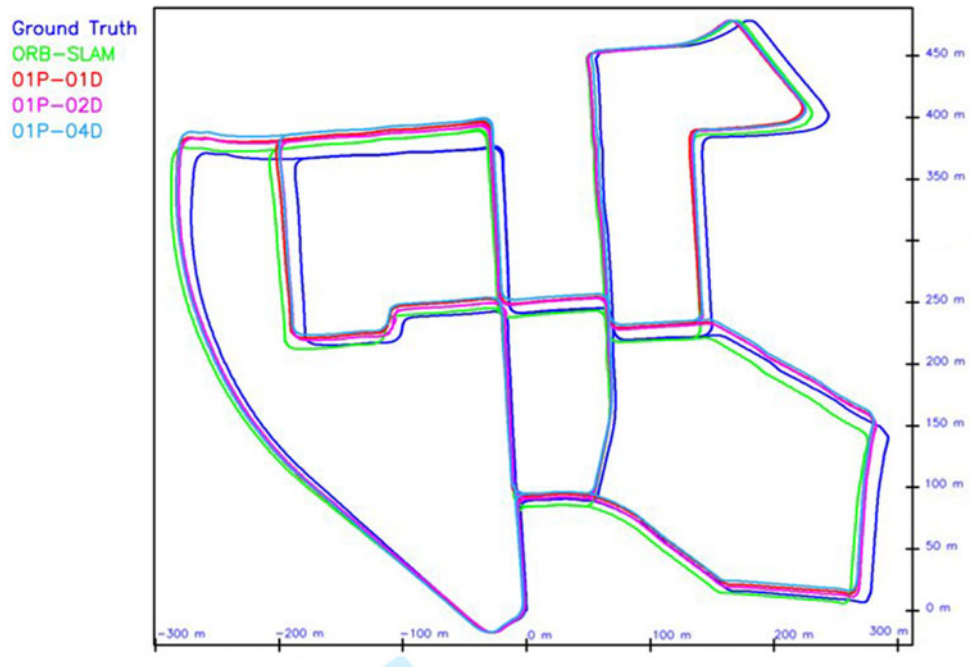
Fig. 16. Map comparison between the reference values for the pose (in blue), calculated using the reference implementation of the ORB-SLAM2 and the modified implementation. The entire system was run on a single machine.
