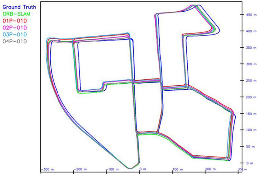
Fig. 21. Comparison of the reference map, that is, the ORB-SLAM2 original version map, and maps created using the modified version of the system running point extraction and descriptor calculation on an i7 3517U i7 processor communicating over Gigabit Ethernet.
