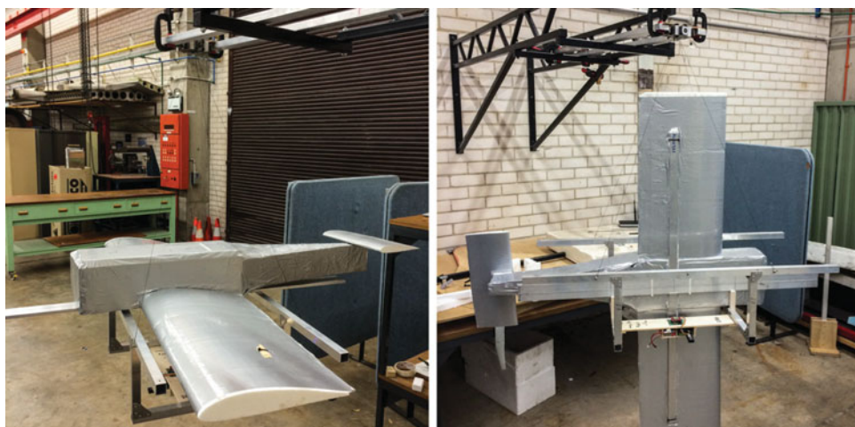
Figure 10. (Colour online) Inertia simulator for the 1DoF case.
