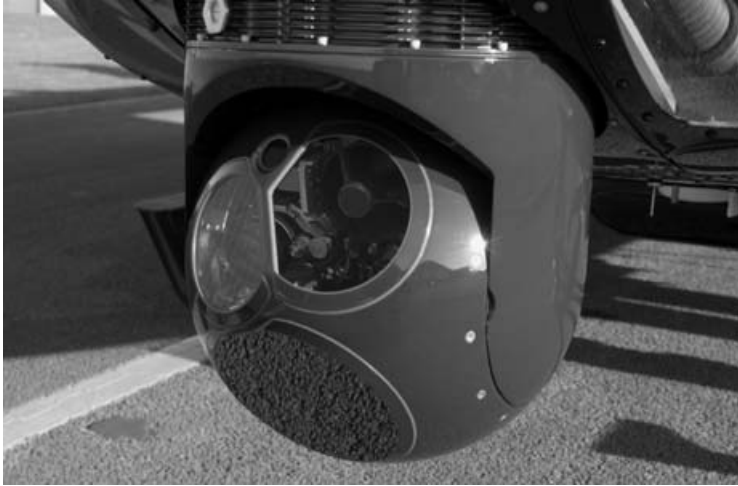
Figure 3. The turret of the WESCAM MX-15 camera.
