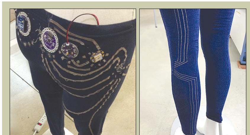
The leggings are made from PA/Lycra knitted fabric that allows it to fit tightly to the body. The circuits are knitted with highly conductive yarn (staten shieldtex 117/17) to connect the external sensors placed on the garment. The quantified walk prototype was manufactured at the Swedish School of Textiles, Delia Dumitrescu and Kristian Rödbý 2017. Team: Felecia Davis, Delia Dumitrescu, Kristian Rödbý. © 2020 Felecia Davis.
