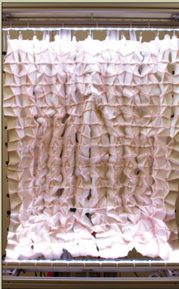
(Left) The Textile Mirror is a prototype wall panel that changes shape in response to people’s emotions. © 2020 Microsoft Research. (Right) A sample using resistive yarns that can be used as a sensor. © Felecia Davis.
