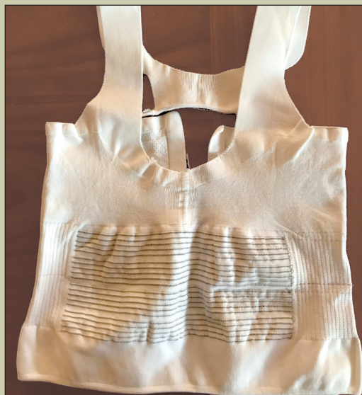
Prototype of the pulmonary fibrosis camisole top. The fabric of the top is tested at Hershey Medical Center. The white yarn (PA/Lycra) is selected because it is lightweight to be worn under other garments, and elastic to make it fit close to the body. The sensor yarn (Bekintex BK 50/2) is resistive and sits under the chest area. When a person’s lungs expand and then contract, they expand and contract the resistive yarn that is connected to a microcontroller that can read the patterns of coughing. For stitching, lace structures are chosen for the sides and back to allow a better thermal circulation, and full rib on the front side for more elasticity and better ability to stretch and recover the original shape. The Team who made the top: Rebecca Bascom, MD, PSU Hershey College; Felecia Davis; and Dr. Dumitrescu of the Swedish School of Textiles. Seen in photo (top left): Erin Lewis, 3rd year PhD student, Swedish School of Textiles (front); then Delia Dumitrescu; Anne Dimmock, 1st year Hershey Medical student (back, left); and Farzaneh Oghazian, 3rd year PhD student, Penn State University, SOFTLAB in the Stuckeman Center for Design Computing. Image credit: Delia Dumitrescu at the Swedish School of Textiles © 2020; Image credit, top right and bottom left: Felecia Davis © 2020.
