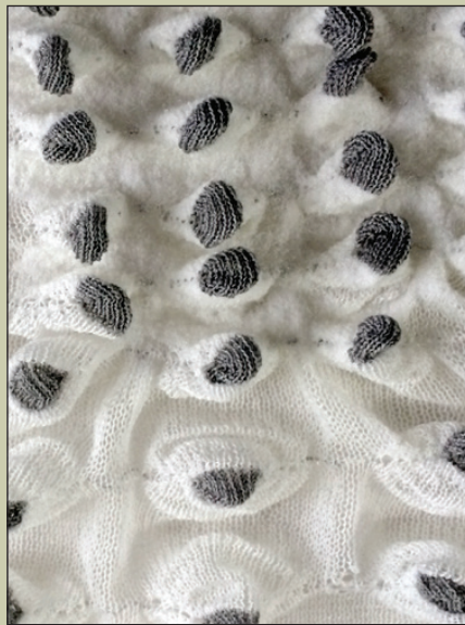
(Left) The Textile Mirror is a prototype wall panel that changes shape in response to people’s emotions. © 2020 Microsoft Research. (Right) A sample using resistive yarns that can be used as a sensor. © Felecia Davis.
