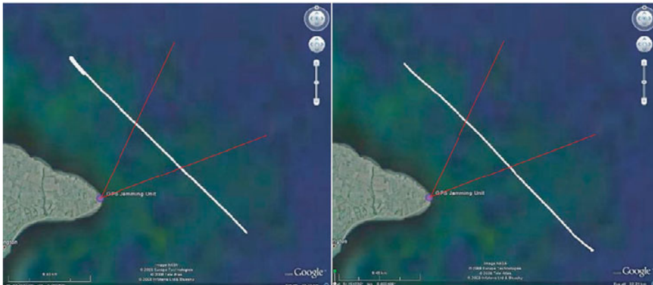
Figure 4. Two plots of eLoran data displayed in Google Earth™. The left-hand plot is the reported positions during a control run when there was no GPS jamming. The right-hand plot shows the reported positions during a run with GPS jamming switched on. The red lines indicate the approximate boundaries of the main lobe of the GPS jamming signal. eLoran was not affected by GPS jamming.
