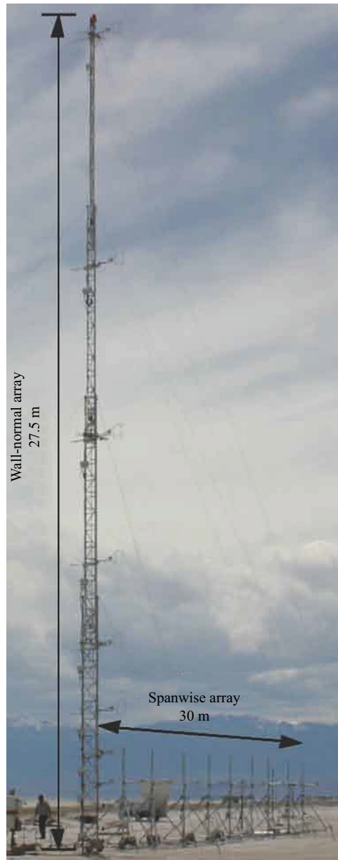
Figure 2. Measurement array installed at the SLTEST site. This figure was adapted from Hutchins et al. (2012) .
