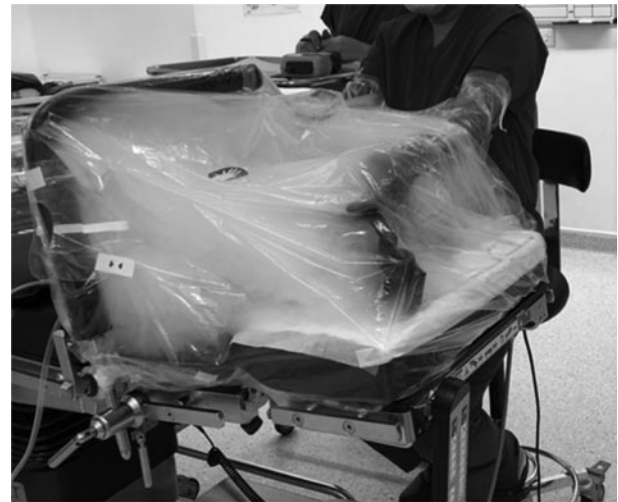
Fig. 2. Smoke generation within the drapes to ensure no visual leaks and a 'tight seal'.
