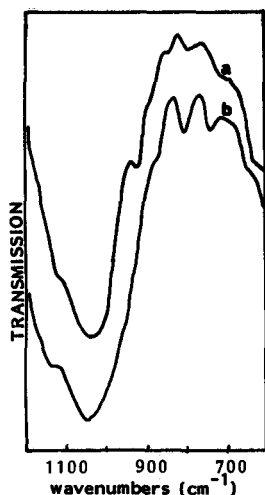
Figure 5. Infrared spectra of the original Greek montmorillonite (a) unheated and (b) heated at 760°C.
