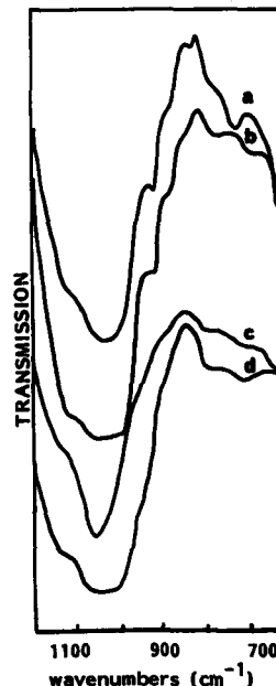
Figure 6. Infrared spectra of the Al-pillared interlayer complex (a) unheated and heated at (b) 300°C, (c) 700°C, (d) 760°C.
