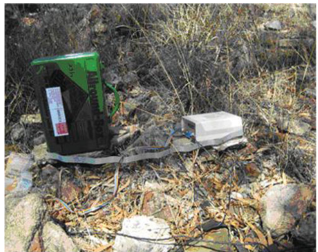
Fig. 6. Mössbauer spectrometer MIMOS II in measuring position. The sensor head can be placed in any direction depending on the sample to be analysed.
