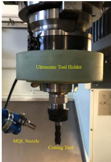
Fig. 2. Ultrasonic tool holder used in experiments.
