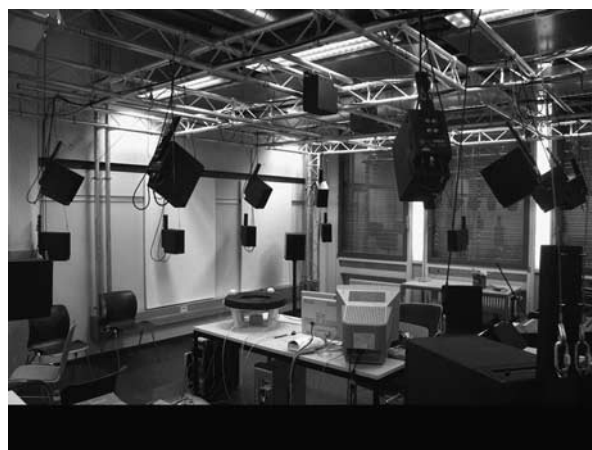
Figure 2. The smaller 24-channel dome in the studio. Photo: Bernhard Sturm © ZKM 2007.
